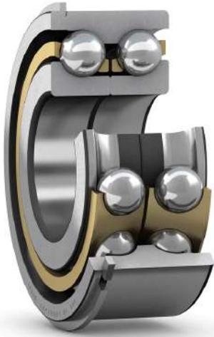
Double row angular contact ball bearings, with snap ring and split inner ring, correspond to a pair of single row angular contact ball bearings in a back-to-back arrangement. The snap ring, fitted in an annular groove in the outer ring, facilitates axial location of the bearings within their housings. The split inner ring enables incorporation of more balls, resulting in higher load carrying capacity.
