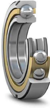
Four-point contact ball bearings with locating slots can accommodate high axial loads in both directions and small radial loads. They can operate at very high speeds and are more suitable than deep groove ball bearings for supporting large axial forces. The outer ring, with ball and cage assembly, can be mounted separately from the two inner ring halves. The locating slots can be used to prevent the outer ring from rotating.
