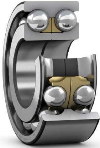
Double row angular contact ball bearings, with two-piece inner ring, correspond to a pair of single row angular contact ball bearings in a back-to-back arrangement, while requiring less axial space than the equivalent pair of single row angular contact ball bearings. The two-piece inner ring enables incorporation of a larger number of balls, with a larger contact angle, providing a high load carrying capacity, especially in the axial direction.
