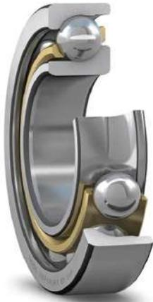
These single row angular contact ball bearings can accommodate radial and axial loads acting simultaneously, where the axial load acts in one direction only. They can operate at high speeds and, depending on the variant, even very high speeds. They are more suitable than deep groove ball bearings for supporting large axial forces acting in one direction.
