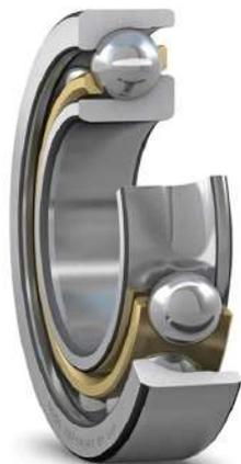
These single row angular contact ball bearings can accommodate radial and axial loads acting simultaneously, where the axial load acts in one direction only. They can operate at high speeds and, depending on the variant, even very high speeds. They are more suitable than deep groove ball bearings for supporting large axial forces acting in one direction.
