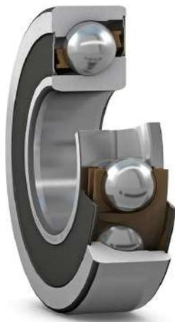
Single row angular contact ball bearing with 40° contact angle and non-contact seals on both sides
