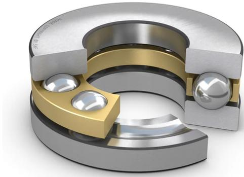
Single direction thrust ball bearings can accommodate axial loads in one direction. They must not be subjected to any radial load. Their separable components facilitate mounting/dismounting and maintenance inspections. Many of the components are interchangeable. The shaft washers have a ground bore that enables an interference fit.
