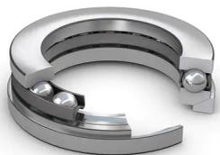
Single direction thrust ball bearings, with sphered housing washer, can accommodate axial loads in one direction. They must not be subjected to any radial load. Many of the components are interchangeable. The shaft washers have a ground bore that enables an interference fit. The sphered housing washers can accommodate initial misalignment when configured correctly with a sphered seat washer or a machine component with a sphered surface.
