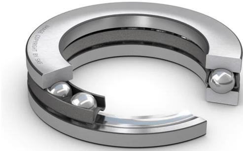
Single direction thrust ball bearings can accommodate axial loads in one direction. They must not be subjected to any radial load. Their separable components facilitate mounting/dismounting and maintenance inspections. Many of the components are interchangeable. The shaft washers have a ground bore that enables an interference fit.
