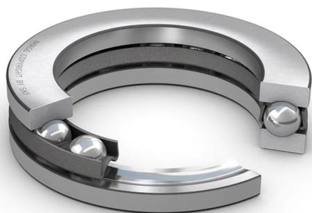
Single direction thrust ball bearings can accommodate axial loads in one direction. They must not be subjected to any radial load. Their separable components facilitate mounting/dismounting and maintenance inspections. Many of the components are interchangeable. The shaft washers have a ground bore that enables an interference fit.
