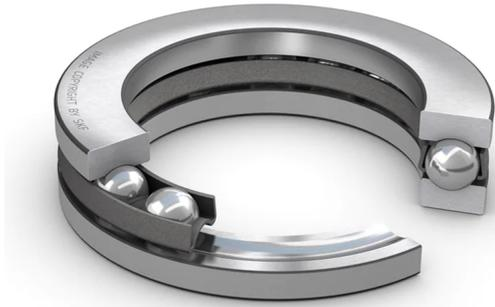
Single direction thrust ball bearings can accommodate axial loads in one direction. They must not be subjected to any radial load. Their separable components facilitate mounting/dismounting and maintenance inspections. Many of the components are interchangeable. The shaft washers have a ground bore that enables an interference fit.
