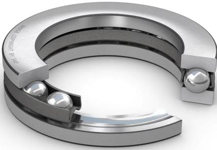
Single direction thrust ball bearings can accommodate axial loads in one direction. They must not be subjected to any radial load. Their separable components facilitate mounting/dismounting and maintenance inspections. Many of the components are interchangeable. The shaft washers have a ground bore that enables an interference fit.
