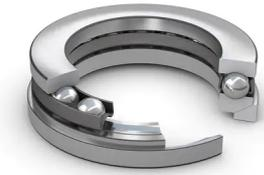
Single direction thrust ball bearings, with sphered housing washer, can accommodate axial loads in one direction. They must not be subjected to any radial load. Many of the components are interchangeable. The shaft washers have a ground bore that enables an interference fit. The sphered housing washers can accommodate initial misalignment when configured correctly with a sphered seat washer or a machine component with a sphered surface.
